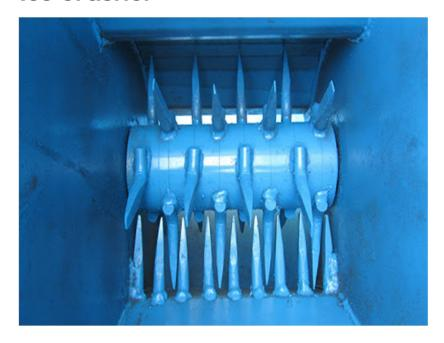
"H.K. Associates" ice Breaker in many application like chemical rections or preserva-tion of perishable goods, ice is used but it has to be broken down into small pieces of about 10 mm to 25 Sizes for best results.
